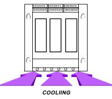
**It is important,** for proper natural convection cooling, avoid to put other objects above the amplifier.
