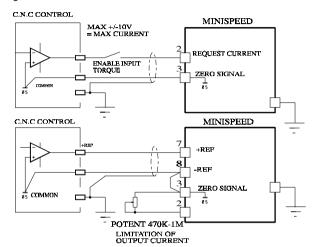
With a "CNC" signal we drive the amplifier in torque mode.
